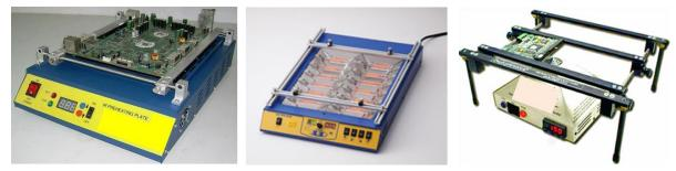
Figure 4. Examples of PCB rework stations with preheater from the bottom
