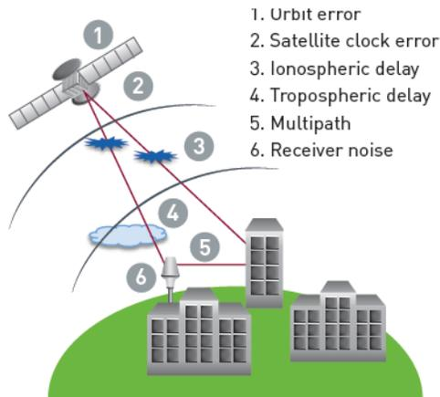
**Multipath:** GPS signals may bounce off of buildings or other obstructions causing delay in the signal.
