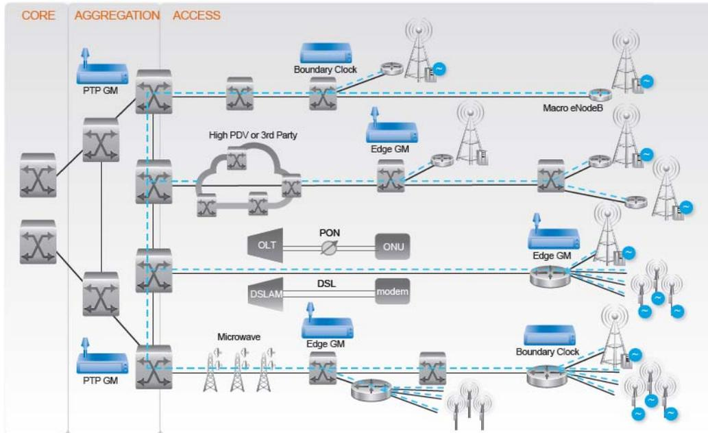
**Figure 6 • Partial On-Path Support and Edge Grandmaster Deployment Scenarios**
