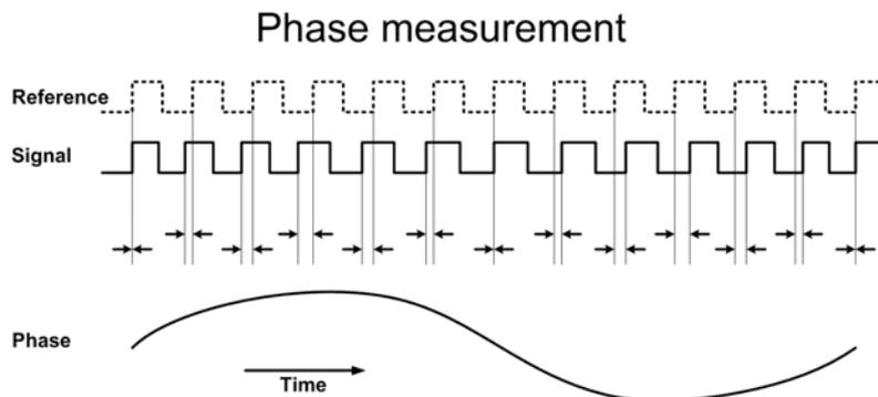
**Fig. 1.** Phase is measured by periodically timing the difference between a reference and the signal and plotting this difference over time.
